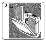
Remove any packaging wrap from the new filters(s) and re-install the filters.
