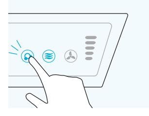
» Ionizer will be off by default. Turn the ionizer on by pressing and holding the ionizer icon until it is illuminated.
