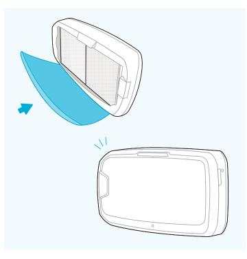
» Place both assembled filters into the unit – white sticker on top and white pre-filter in front.
